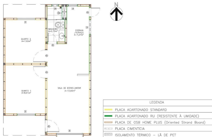
Figura 47 – Planta Light Steel Frame
